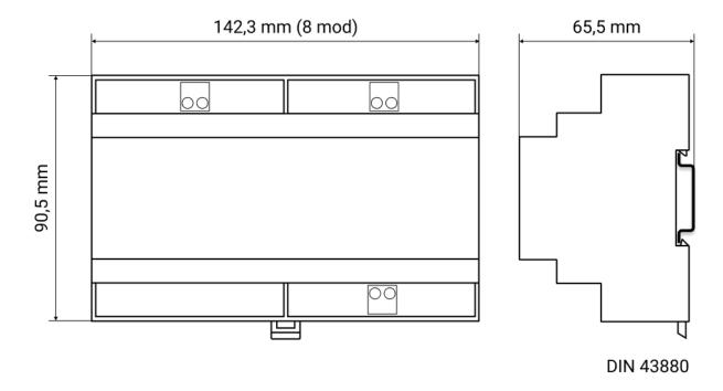
Install in the switchgear, on a horizontal TH35 rail (EN60715) ensuring cooling air circulation. The heat gains generated by the gateway increase with the number of connected M-Bus meters and the frequency of their polling. Installing directly next to other heat emitters, limiting air circulation around and through the gate, or covering the ventilation holes in the housing may lead to overheating, reducing the durability of the device.
